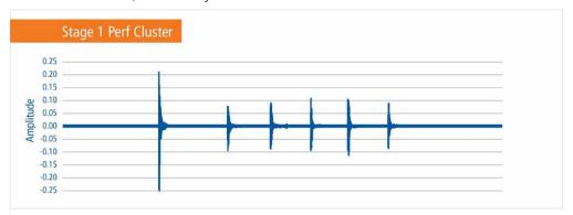
6 detonations in a perforation cluster captured by Retina (pressure data removed for clarity).
