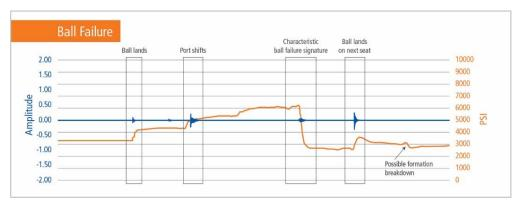
Characteristic ball failure signature, followed by indication of ball landing on the next seat.
