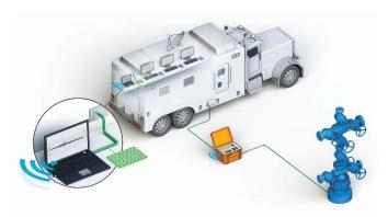
Connectivity between the wellhead, Retina data acquisition box, data van, and Retina laptop.
