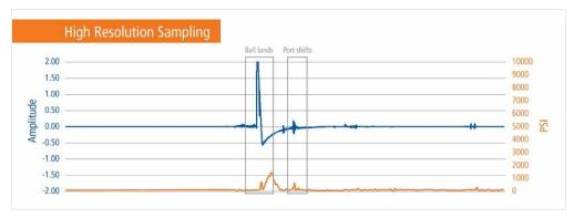
Retina shows the ball landing on seat and shifting, both within 0.4 seconds. The pressure signature was not seen in the data van.
