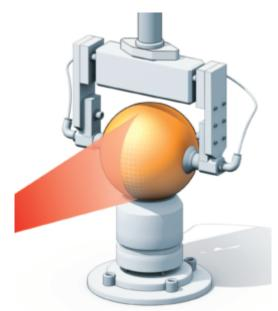
As part of a fully integrated QA/QC process, every ball is inspected with lasers in over 10 positions to check for surface defects, ovality, dimension, etc.
